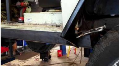
Marking Rail for trimming to fit flare. Make sure front and rear of Rail are parallel with the door opening and not leaning to the front or rear.
